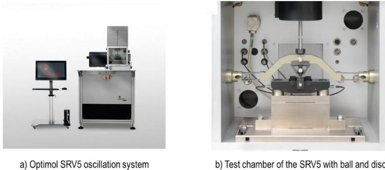
Figure 1. Optimol Instruments SRV5 tribometer for friction and wear testing of diverse materials, surfaces and lubricants (courtesy of Optimol Instruments Prüftechnik GmbH)
