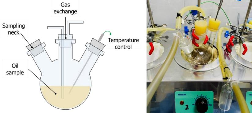
Figure 3. Revised thermal-cycling rig for controlled engine oil aging experiments, with three-neck round bottom flasks and improved control system
