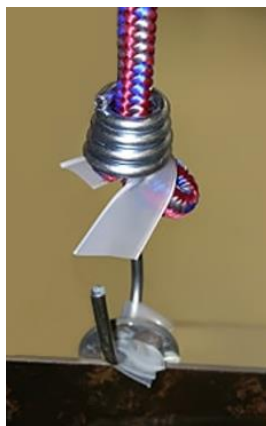
Figure 44: Silicone insert was used between the hook and washer to avoid the metal-metal friction.
